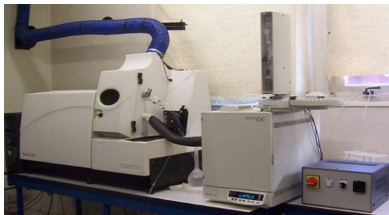
GC-ICP-MS: Focus GC & Thermo X series
