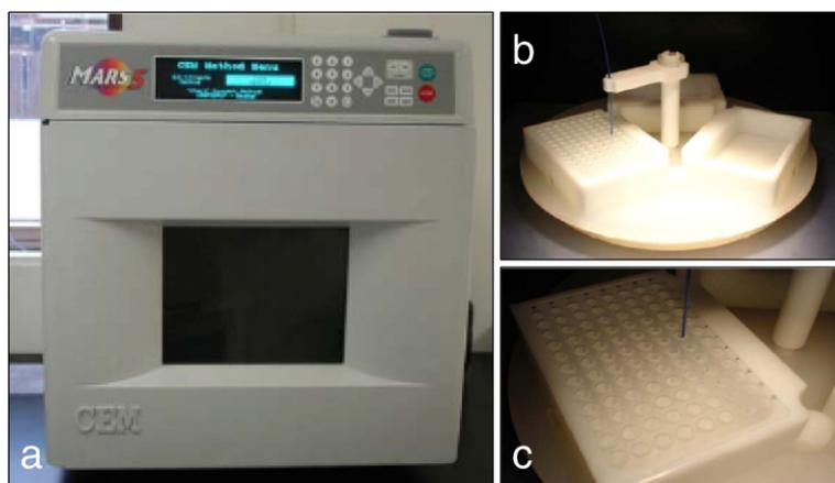
**Fig. 5.** CEM MARS microwave instrument. a, exterior image, b and c, interior images; the turntable designed to hold three 96-well plates (b), and the fiber optic temperature probe inserted in a 96-well PCR plate (c).
