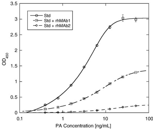
**Fig. 2.** Effect of rhMABs on PA standard curves. Serial dilutions of PA with concentration ranging from 0.39 through 50 ng/mL were tested in duplicate, in the presence of rhMAB1 (□) or rhMAB2 (◇) at constant concentration of 0.2 mg/mL or in the absence of any rhMAB (○). The curves were plotted using the 5-parameter curve fitting function of software SoftMaxPro (Molecular Devices, Sunnyvale, CA).
