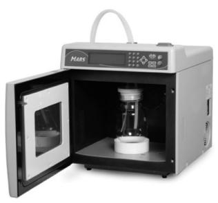
Figure 2. Flow-through reactor (2 L) inside the microwave cavity.
