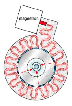
Microwaves couple directly with the molecules present in the reaction mixture, leading to a rapid rise in temperature and increasing the reaction rate.
