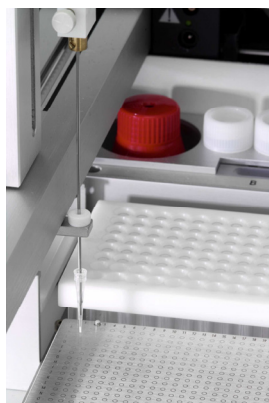
Fig. 2: StageTip on steel needle over target
